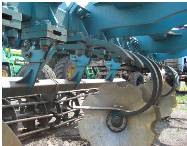
Fig. 1. Destruction of disk spring tines
